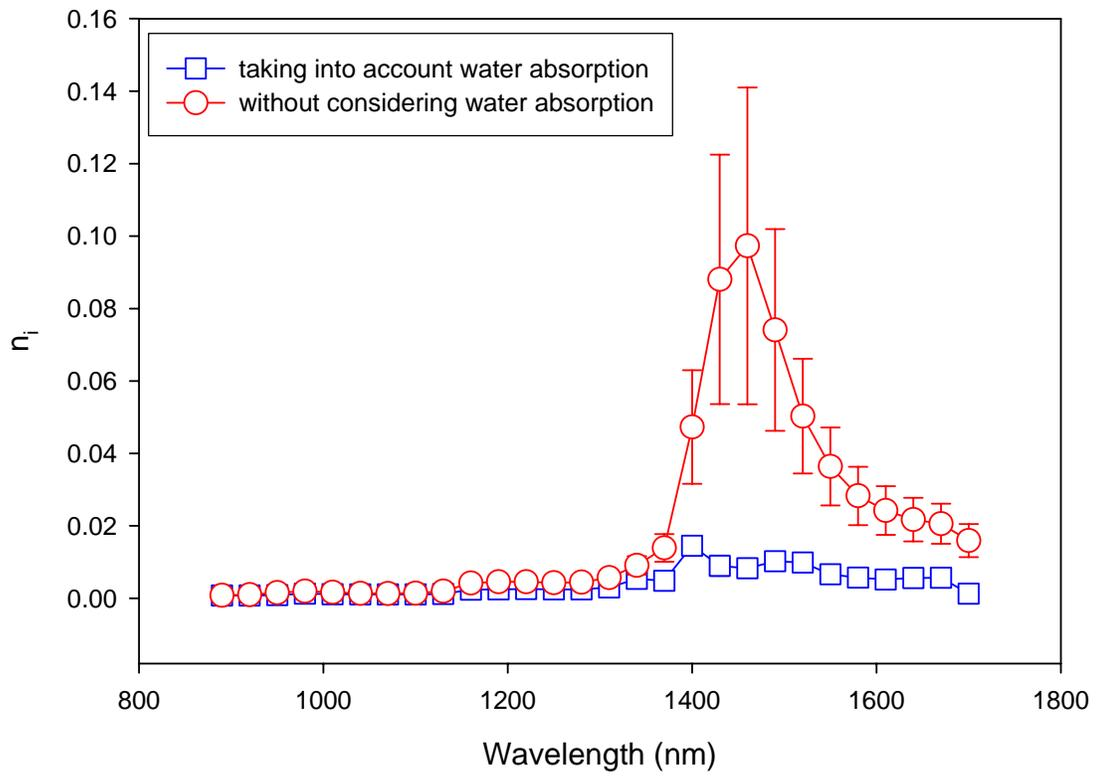
Figure 2.2 Effect of water absorption on the determination of the imaginary refractive index  $n_i$  of polystyrene microsphere. Solid lines are for guide of eye.
