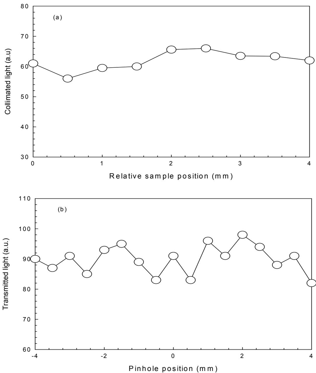
Figure 5.5 (a) the collimated transmission for a porcine dermis sample of 0.54 mm thick at different lateral positions and (b) the light intensity distribution on the focal plane.
