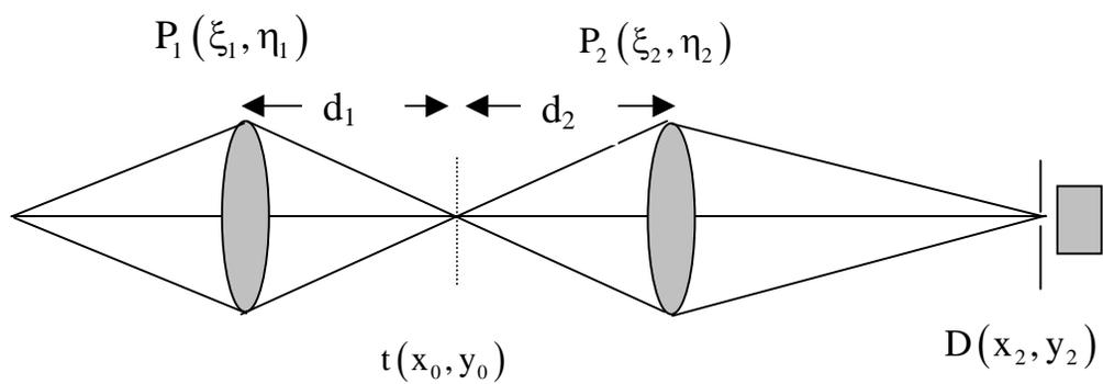
Figure 2.7 Confocal imaging.
