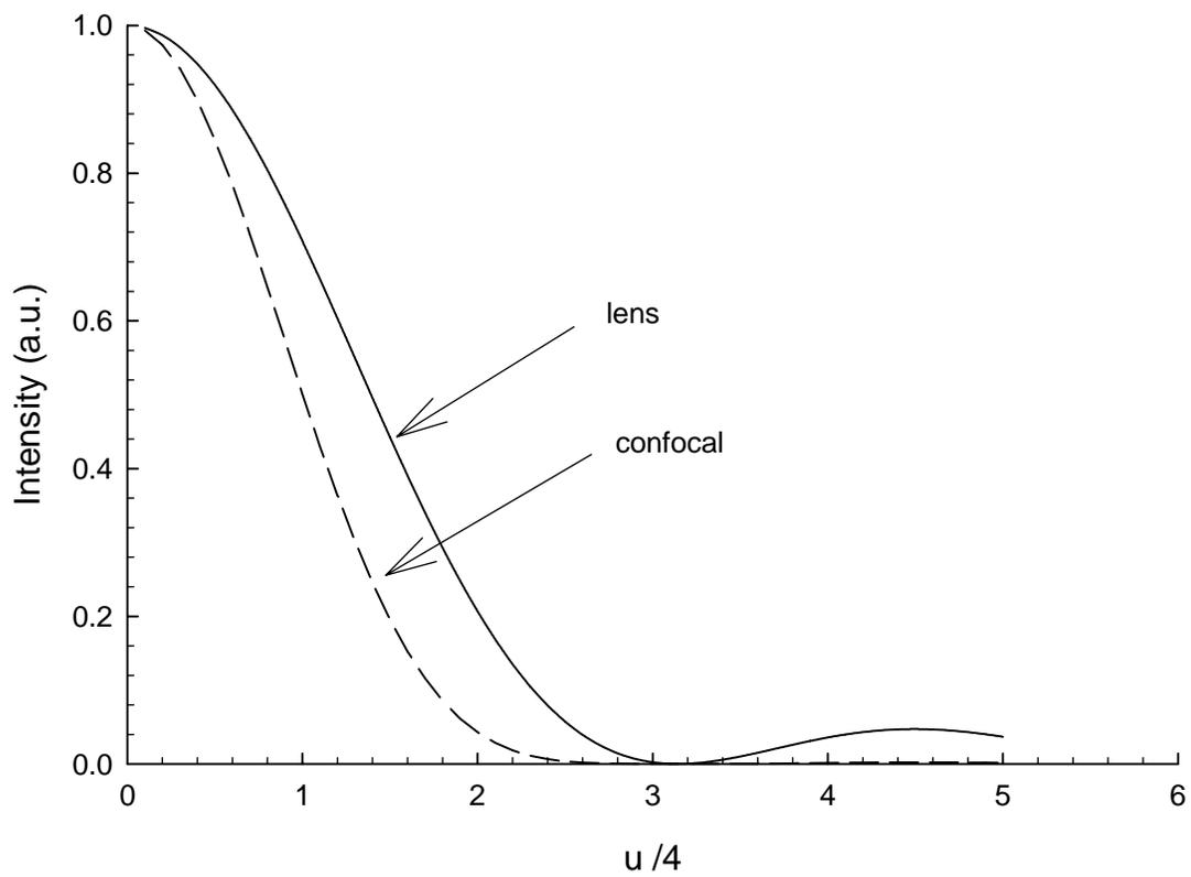
Figure 2.8 Variation of image intensity along the optical axis for conventional lens imaging (solid line) and confocal imaging (dash line).
