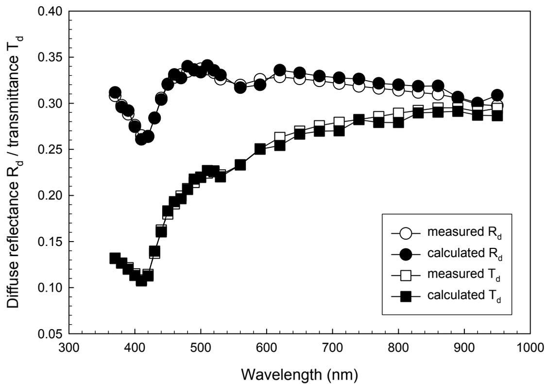
Figure 5.16 Comparison between the calculated and the measured values of  $R_d$  and  $T_d$  for sample of 1.154 mm thick. The solid lines are for guide of the eye.
