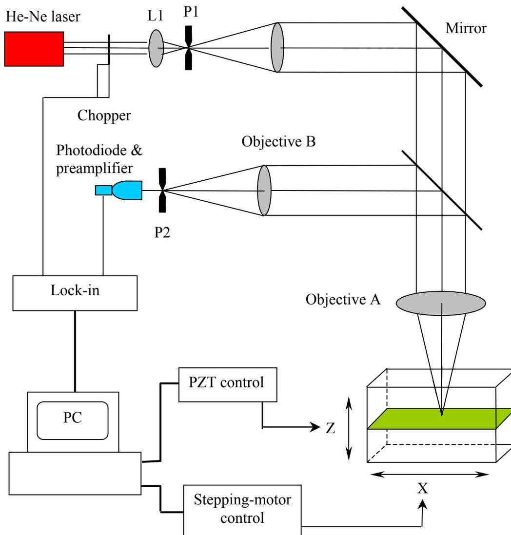
Figure 4.11 Schematics of the scanning confocal imaging system. P1 is a 100  $\mu\text{m}$  pinhole, P2 is a 10  $\mu\text{m}$ ; Not shown above, the sample is mounted on the top surface of PZT and PZT is placed on a translation stage moved by a stepping motor.
