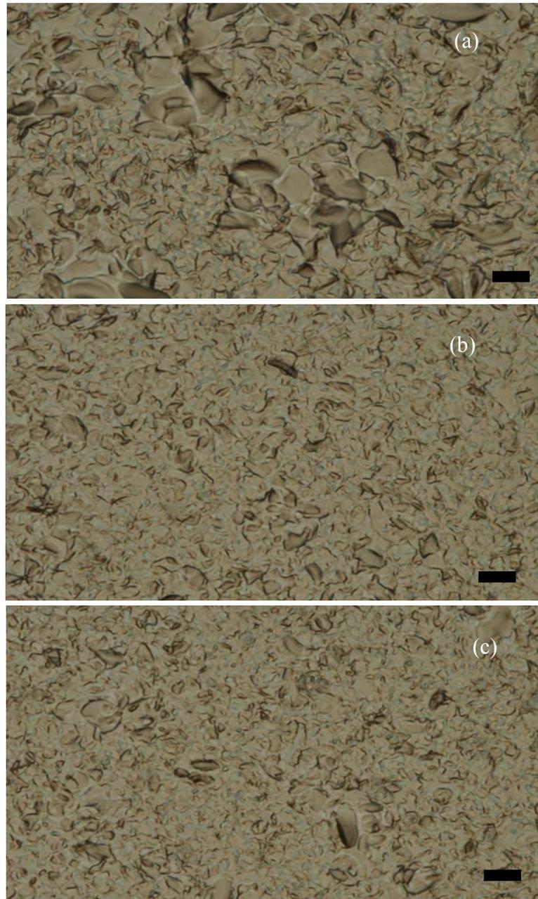
Figure 5.20 Digital microscope images of rough surfaces of glasses grounded with (a) 9.5  $\mu\text{m}$ , (b) 5  $\mu\text{m}$ , and (c) 3  $\mu\text{m}$  polishing powder. The black bar in each graph represents 10  $\mu\text{m}$  long.
