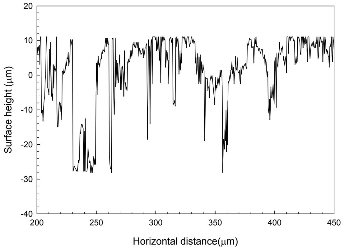
Figure 5.22 A line surface profile for a rough surface with  $\delta = 10.39$   $\mu\text{m}$  and  $a = 8.10$   $\mu\text{m}$ .
