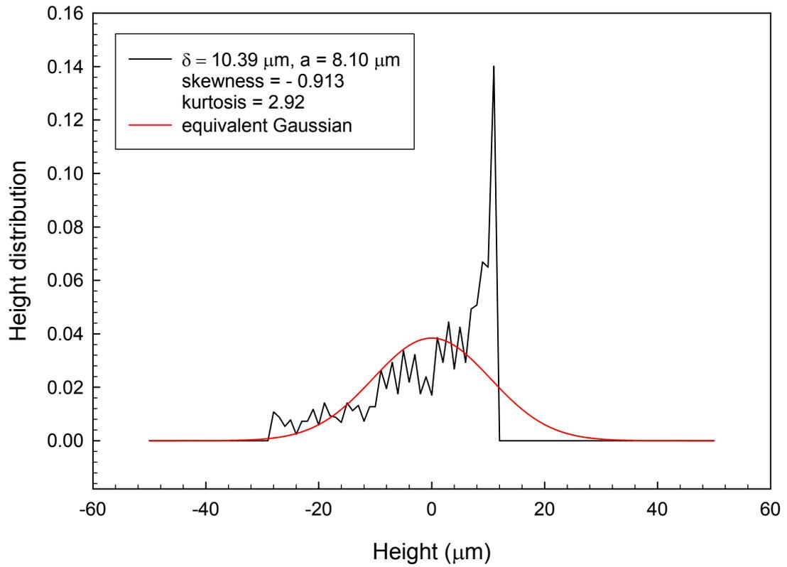
Figure 5.23 Surface height distribution function (black line) with its equivalent Gaussian function (red line) for a rough surface profile.
