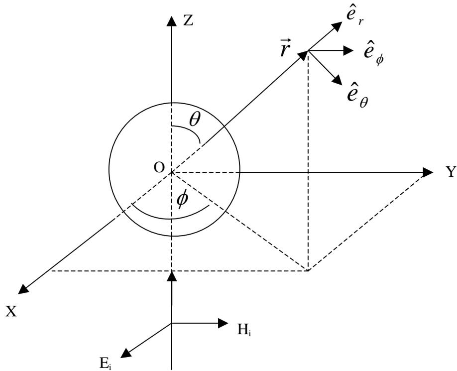
Figure 2.1 Geometry for the scattering of a linearly polarized plane wave by a spherical particle.
