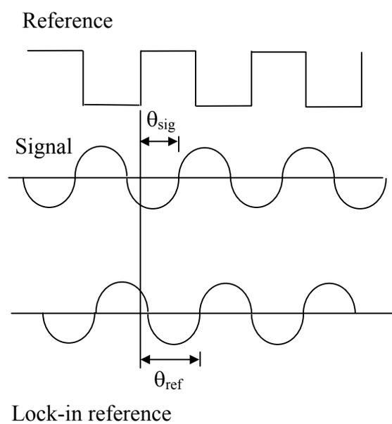
Figure 4.9 Relationship between the reference signal, signal, and the lock-in reference.
