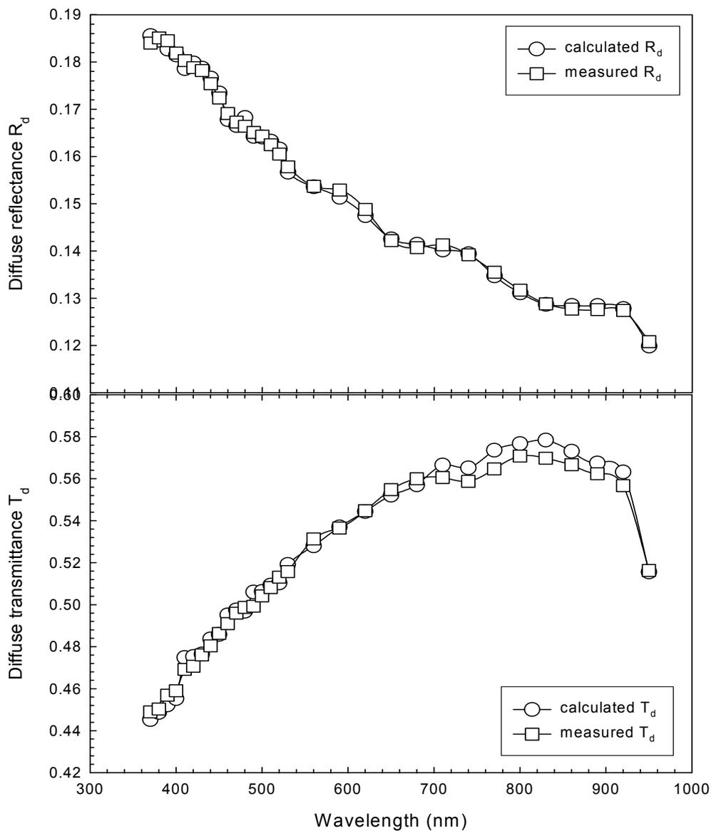
Figure 5.11 Comparison between the calculated and measured (a)  $R_d$  and (b)  $T_d$  for a polystyrene suspension with a concentration of  $1.569 \times 10^6 \text{ mm}^{-3}$ . Solid lines are for guide of eye.
