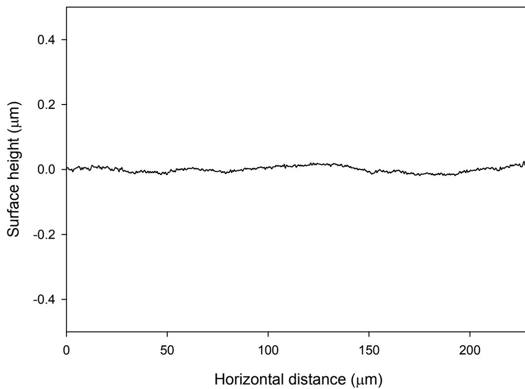
Fig 5.25 Surface profile for an optical flat window glass reconstructed by confocal imaging.
