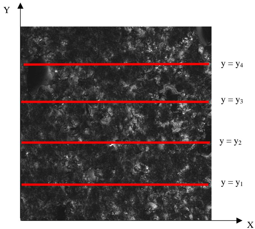
Figure 3.2 The schematic diagram to show how the one-dimensional line surface profiles are chosen to perform the statistical analysis.
