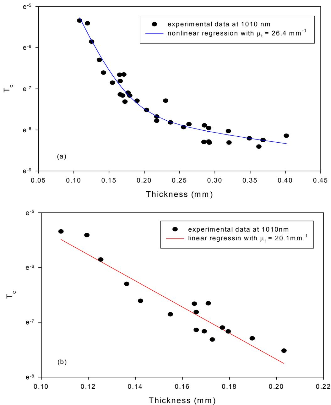
Figure 5.14 Comparison between linear regression and nonlinear regression for the determination of  $\mu_t$  from  $T_c$ .  $T_c$  is plotted in ln scale.
