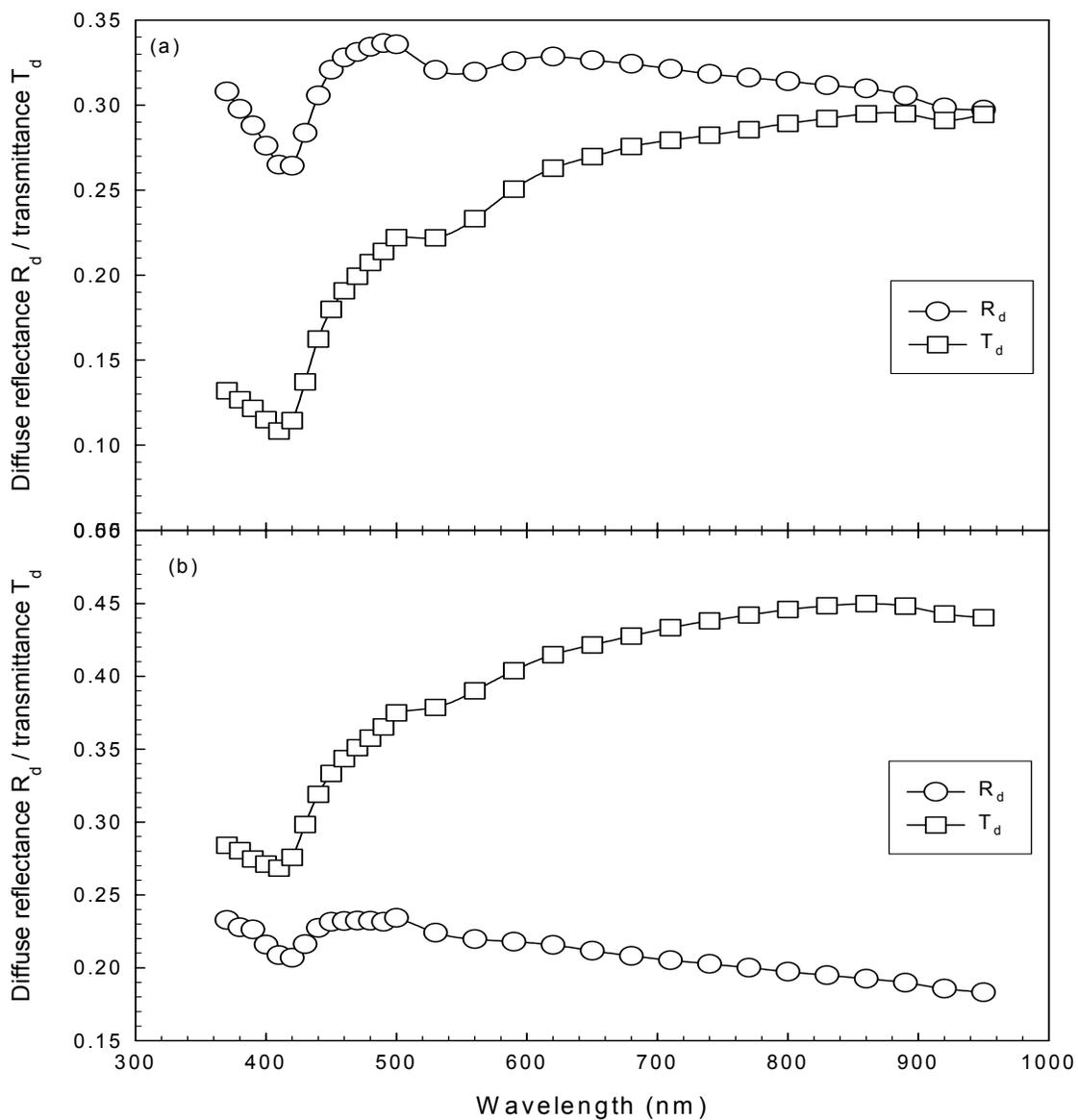
Figure 5.12 Diffuse reflectance  $R_d$  and transmittance  $T_d$  of two porcine dermis samples with thickness of (a) 1.15 mm and (b) 0.56 mm. The solid lines are for guide of the eye.
