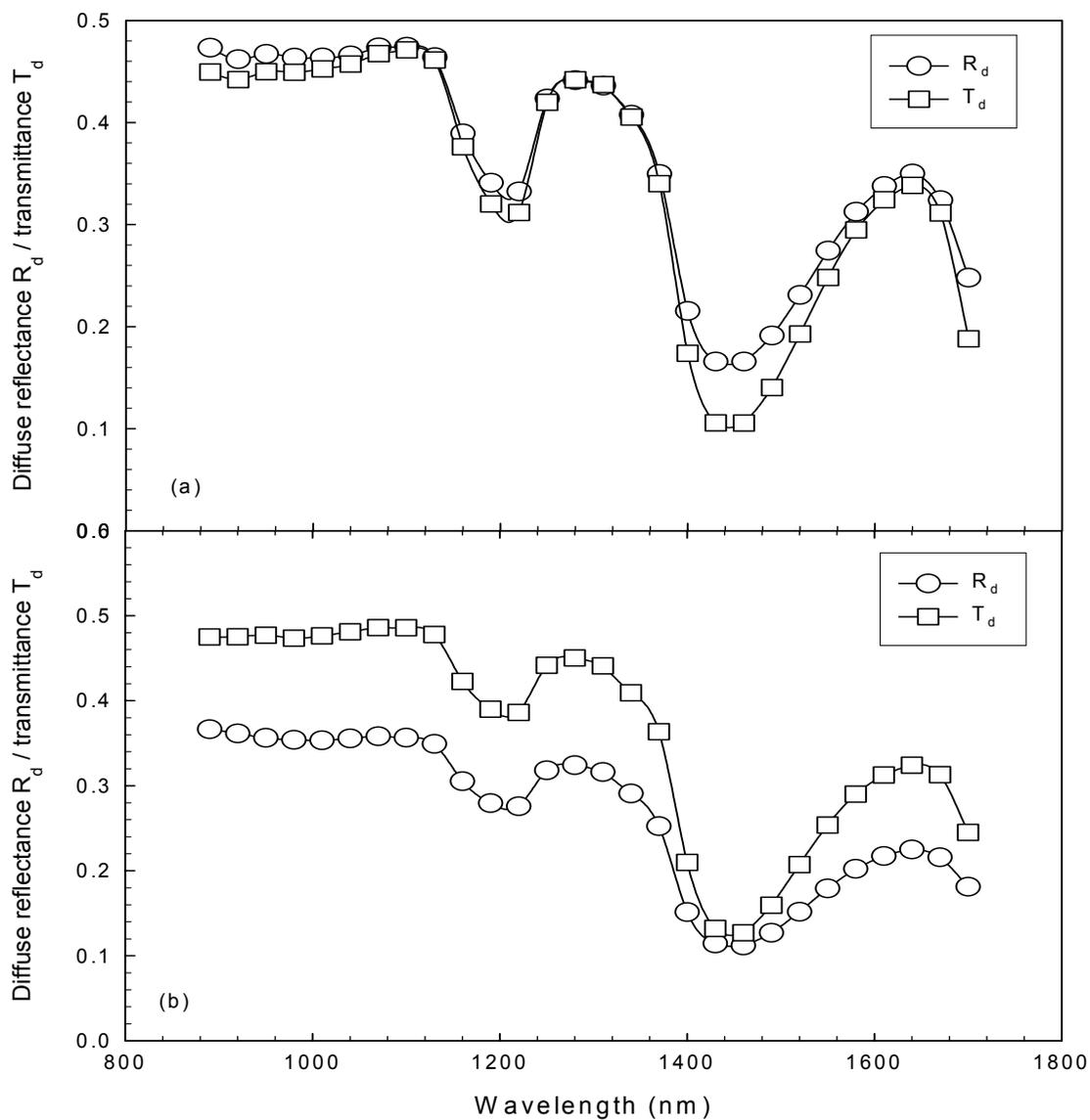
Figure 5.13 Diffuse reflectance  $R_d$  and transmittance  $T_d$  for two porcine dermis samples with thickness of (a) 1.07mm and (b) 0.65mm. The solid lines are for guide of the eye.
