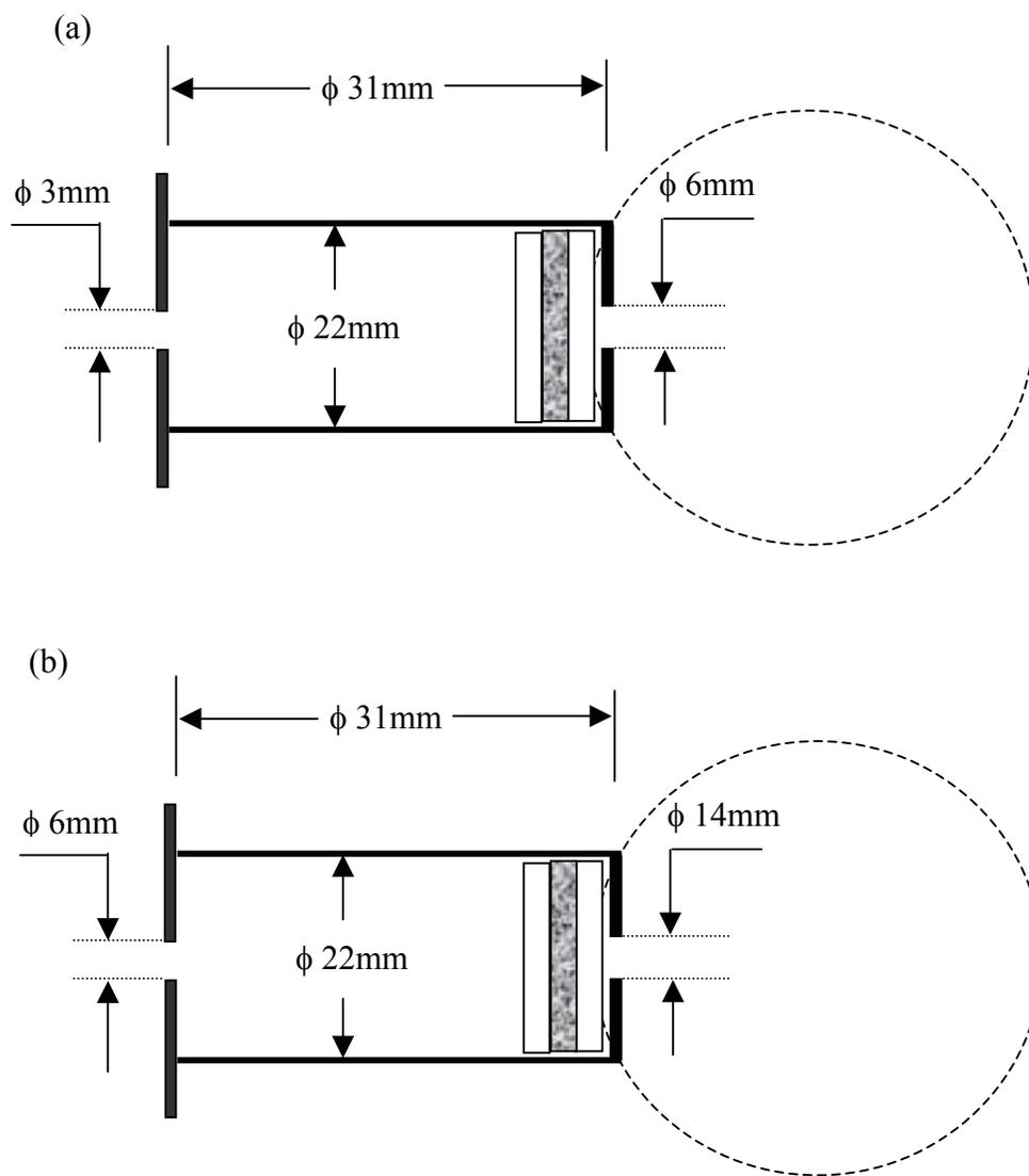
Figure 4.7 Sample holders for integrating sphere: (a) for  $R_d$ ,  $T_d$ , and  $T_c$  from the same sample; (b) for  $R_d$  and  $T_d$  only.
