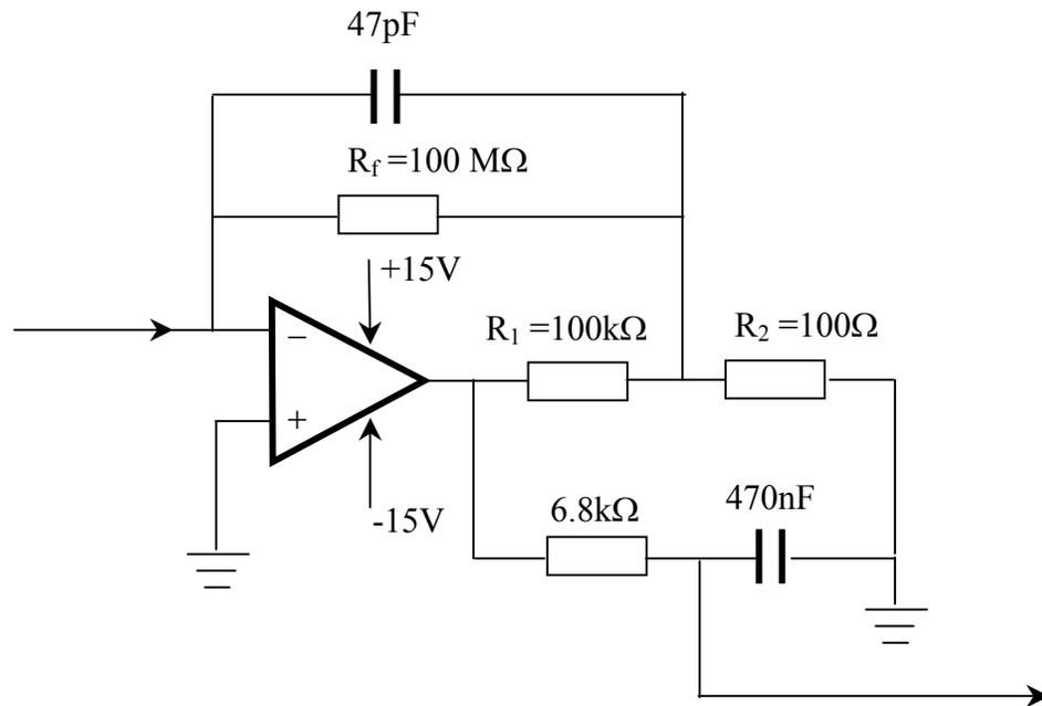
Figure 4.8 Circuit of preamplifier.
