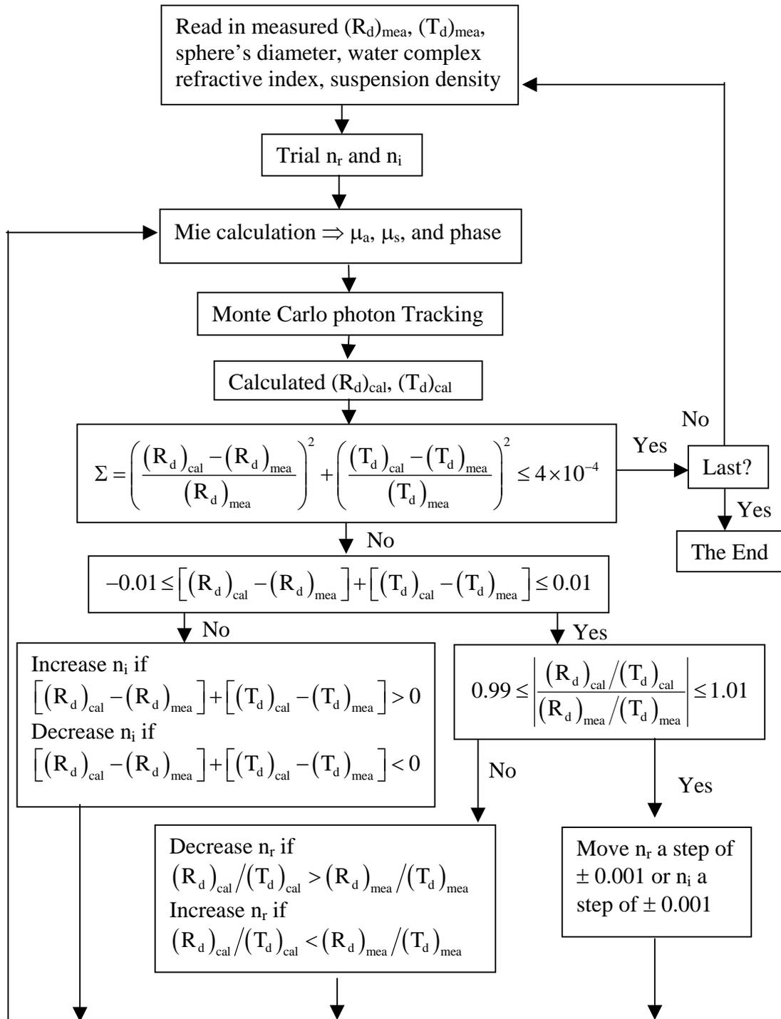
**A.5 Flow Chart of Monte Carlo Based Manual Determination of  $\mu_s$ ,  $\mu_a$ , and  $g$  under rough surfaces from  $R_d$ ,  $T_d$ , and  $T_c$**
