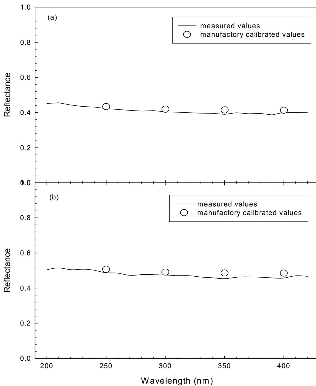
Figure 5.2 Calibration of integrating sphere setup with two reflectance standards: (a) 40% and (b) 50%.
