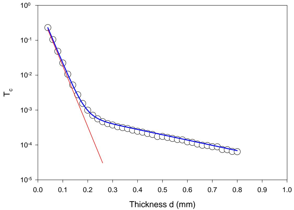
Figure 2.4 Dependence of collimated transmission  $T_c$  on thick  $d$ . Circles represents Monte Carlo simulated  $T_c$  with  $\mu_a = 0.4 \text{ mm}^{-1}$ ,  $\mu_t = 40 \text{ mm}^{-1}$  and  $g = 0.8$ . The red line shows the decay of  $\exp(-\mu_t \cdot d)$ . The blue line represents function
