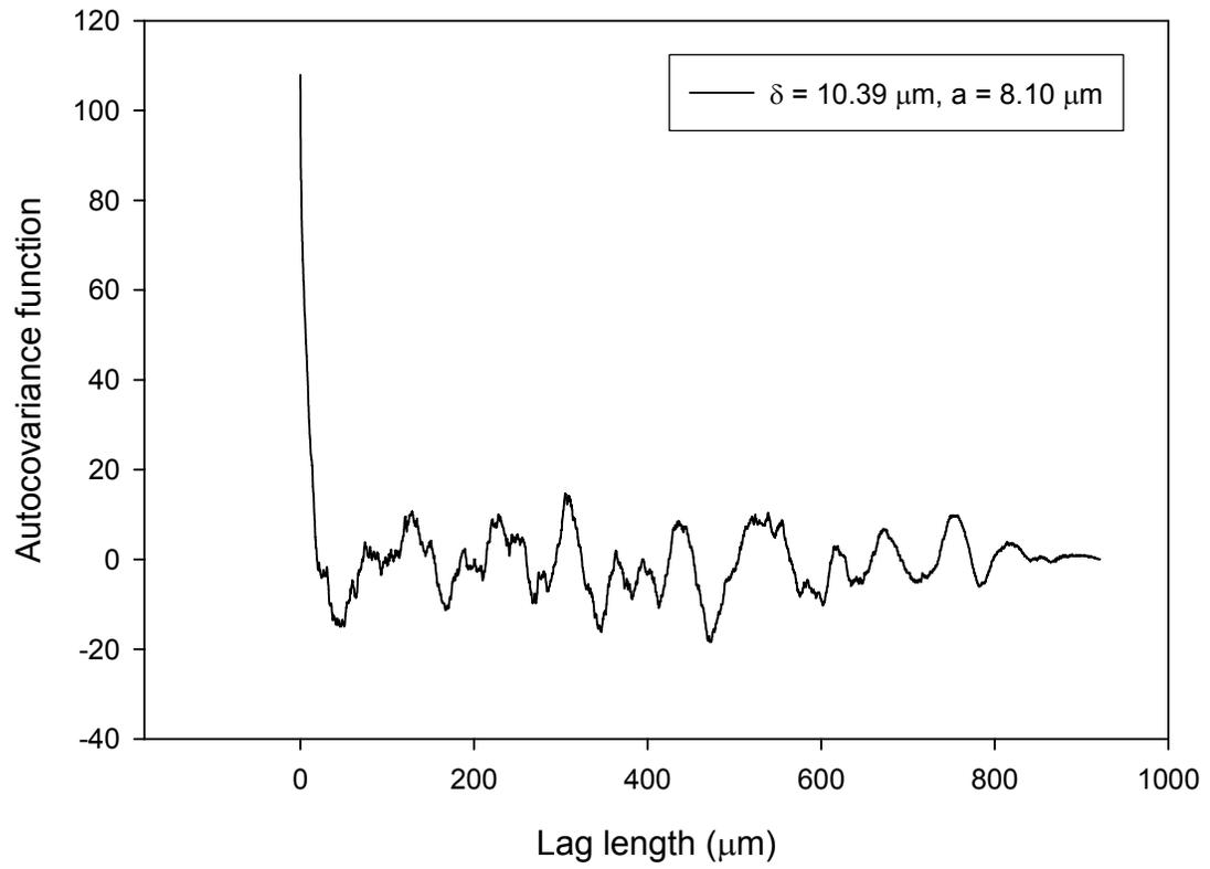
Figure 5.24 Autocovariance function for a rough surface with  $\delta = 10.36 \mu\text{m}$  and  $a = 8.10 \mu\text{m}$ .
