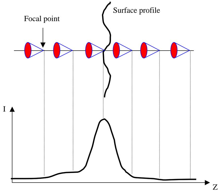
Figure 3.1 The schematic diagram that illustrates the relationship between the reflected light intensity  $I$  recorded by a confocal microscope and the focal point position of the confocal microscope relative to the rough surface.
