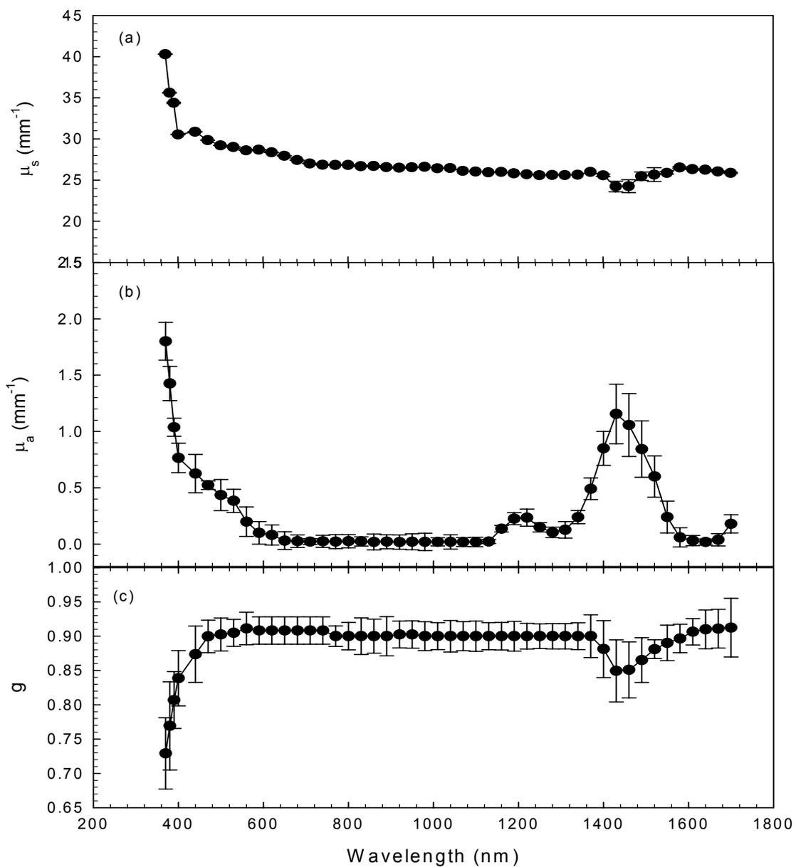
Figure 5.15 The average values of the optical parameters determined under smooth surface assumption for porcine dermis tissue. The error bars represent the standard deviation among 10 samples. The solid lines are for guide of eye.
