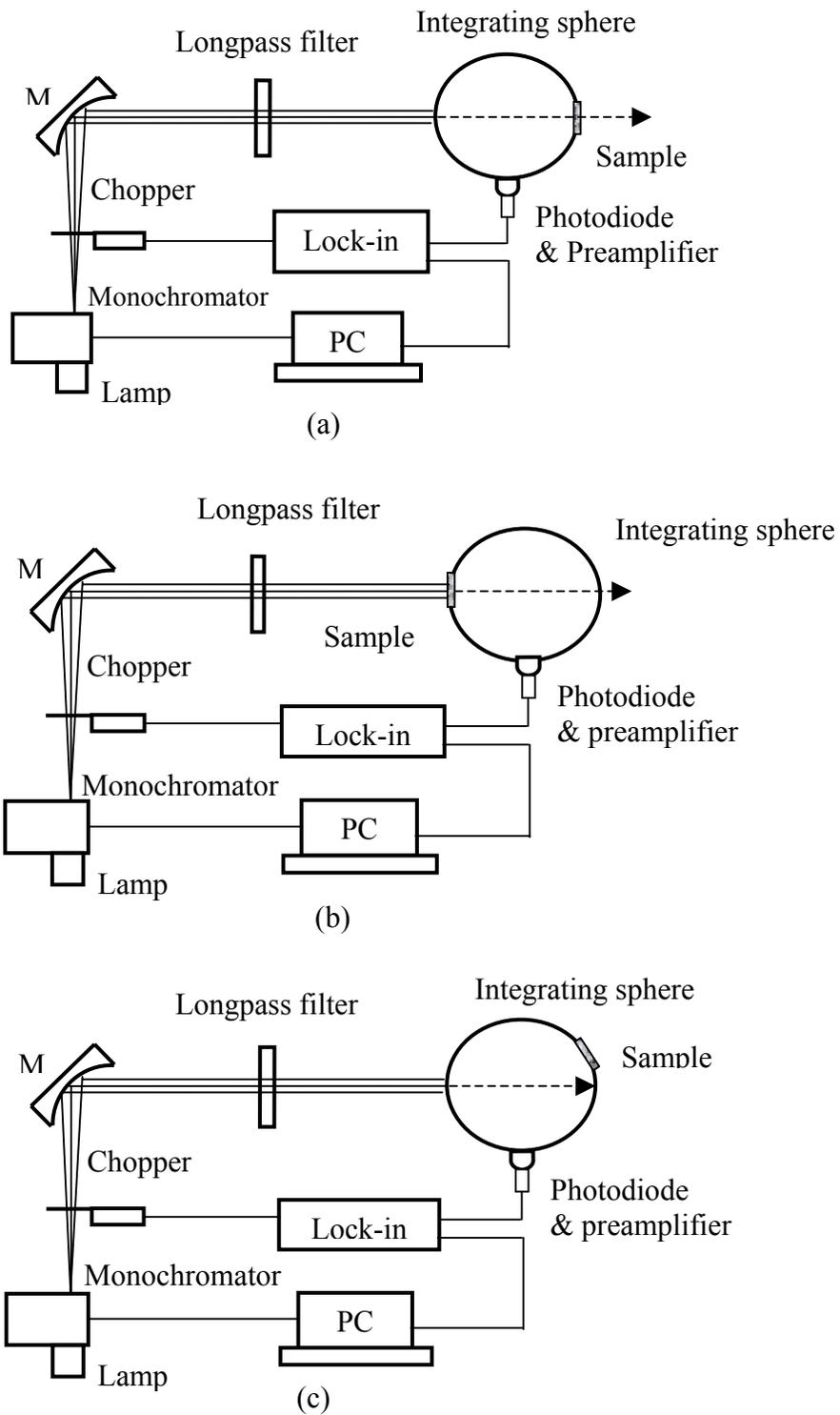
Figure 4.2 Schematics for measurement of (a) the diffuse transmittance  $T_d$  and (b) the diffuse reflectance  $T_d$  and (c) the reference.
