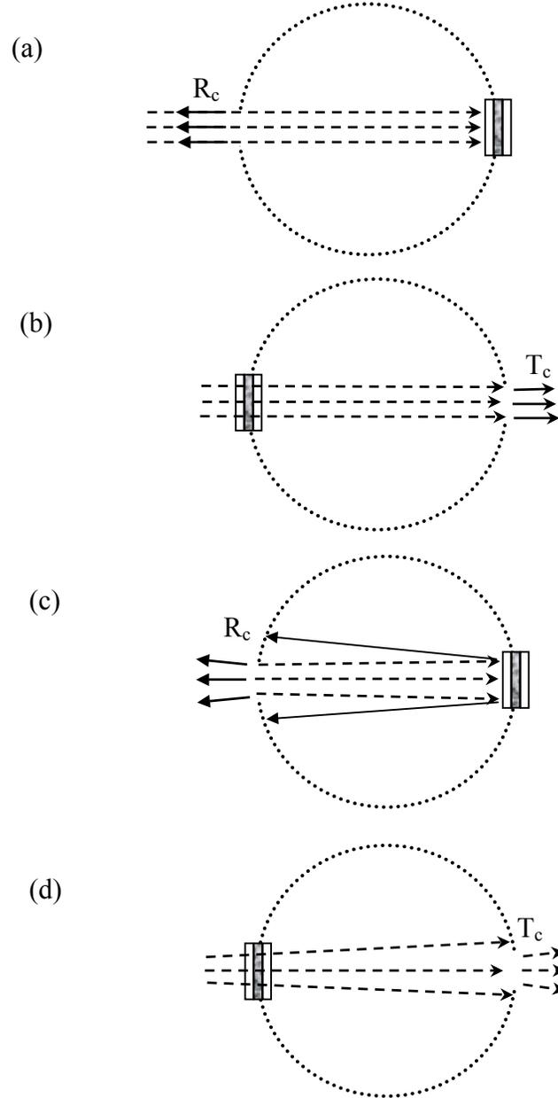
Figure 4.3 Differences between collimated incident beam and diverged incident beam. (a) and (b) are the collimated incident beam for the specular reflection  $R_c$  and the collimated transmission  $T_c$  respectively; (c) and (d) are the diverged incident beam for the specular reflection  $R_c$  and the collimated transmission  $T_c$  respectively.
