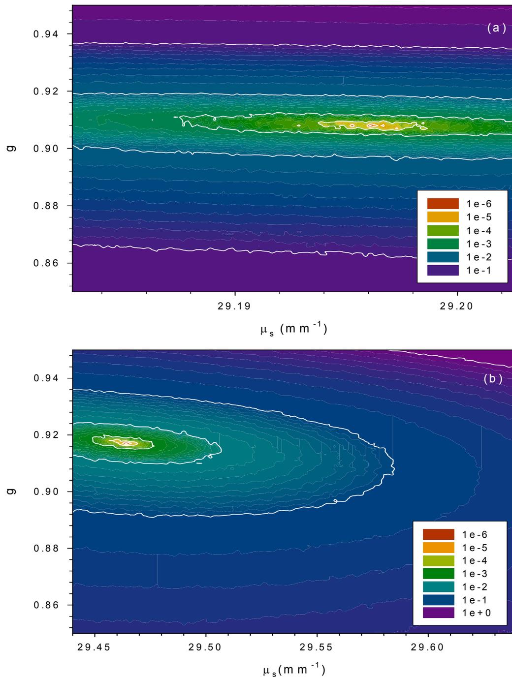
Figure 5.17 Contour plot of the error function  $\Sigma$  in the plane of  $\mu_s$  and  $g$  for porcine dermis sample of 0.246 mm thick at (a) 500 nm and (b) 1460 nm.
