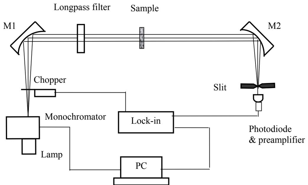
Figure 4.4 Experimental setup for measurement of the collimated transmission  $T_c$  with two concave mirrors M1 and M2.
