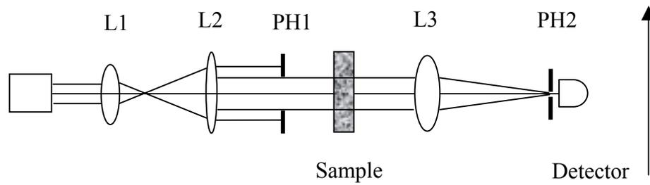
Figure 4.5 Experimental setup to investigate the speckle effect in Tc measurement. L1 and L1 are two convex lenses to expand the laser beam; PH1 is an aperture with a diameter of 2.5 mm; L3 is light collecting convex lens with a focal length of 100 mm; PH2 is a pinhole with diameter of 1 mm. Both sample and detector set (detector plus pinhole PH2) can move in the lateral direction shown as arrow in graph.
