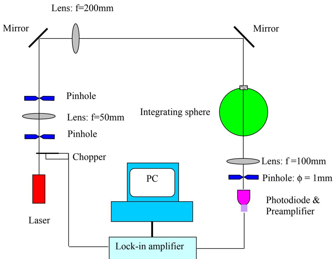
Figure 4.6 Experimental setup for measurements of  $R_d$ ,  $T_d$  and  $T_c$  on a same sample.
