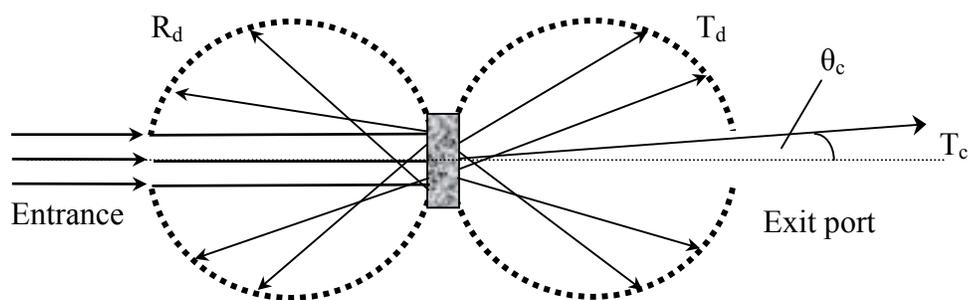
Figure 4.1 Diagram showing the definitions of the diffuse reflectance  $R_d$ , the diffuse transmittance  $T_d$  and the collimated transmission  $T_c$ .
